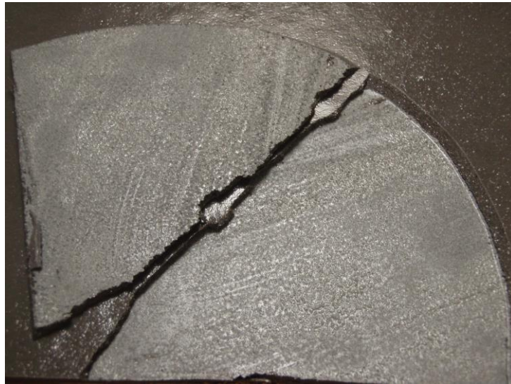
Figure 4 Resin Rich Blister, Wet and Gummy to touch
