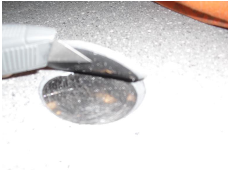
Figure 2: Delamination caused by Rust
